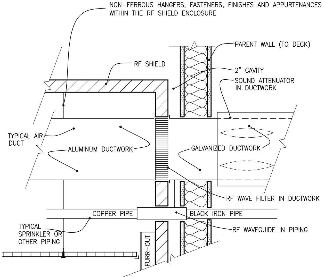
NOTE: RF WAVEGUIDES AND FILTERS FURNISHED AND INSTALLED BY RF SHIELDING SUPPLIER. DUCTWORK, PIPING, WIRING AND CONDUIT INSTALLATION MUST BE CAREFULLY COORDINATED BETWEEN CONTRACTOR'S FORCE AND THE RF SHIELD VENDOR, IN ACCORDANCE WITH THE MRI MANUFACTURER'S SITE PREPARATION REQUIREMENTS.
